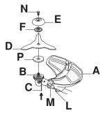
Screw the support cup (E) onto the output shaft threads (CAUTION! Left-hand thread). Tighten to a torque of 35-50 Nm (3.5-5.0 kpm). Use the socket spanner in the tool kit. Note that the locking pin (C)
